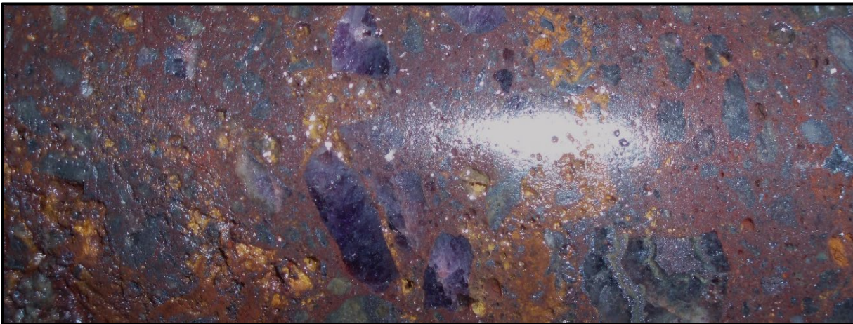
VG-025: polymictic breccia with silica-hematite cement containing fragments of amethyst quartz vein and banded vein
