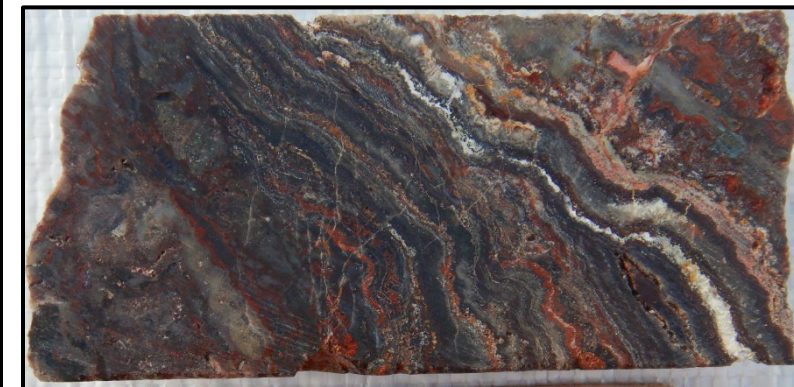
Banded colloform greenish-gray epithermal quartz vein with fine-grained sulfides (Galena) and silica-hematite veinlets, at a depth of 58.85 m
