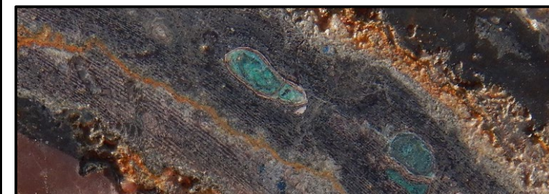
Copper oxides filling voids in the main vein-breccia structure.
