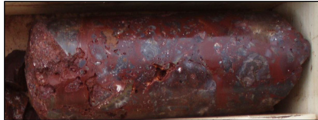
VG-036: breccia with silica-hematite cement containing fragments of vein and previous silica-hematite breccia
