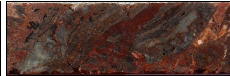
Banded greenish-gray quartz vein, silica-hematite veinlets cutting the first-stage epithermal vein; at a depth of 52.5m.
