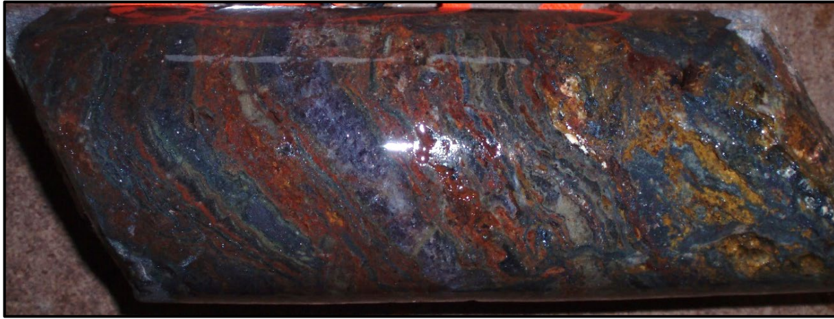
VG-025: vein with bands of greenish cryptocrystalline quartz, sil-hem, microcrystalline amethyst quartz, fine sulfides (gln+sph).
