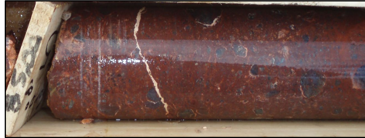
VG-068: polymictic hydrothermal breccia (vein fragments >> host rock fragments) with silica-hematite cement cut by white clays fracture fillings.
