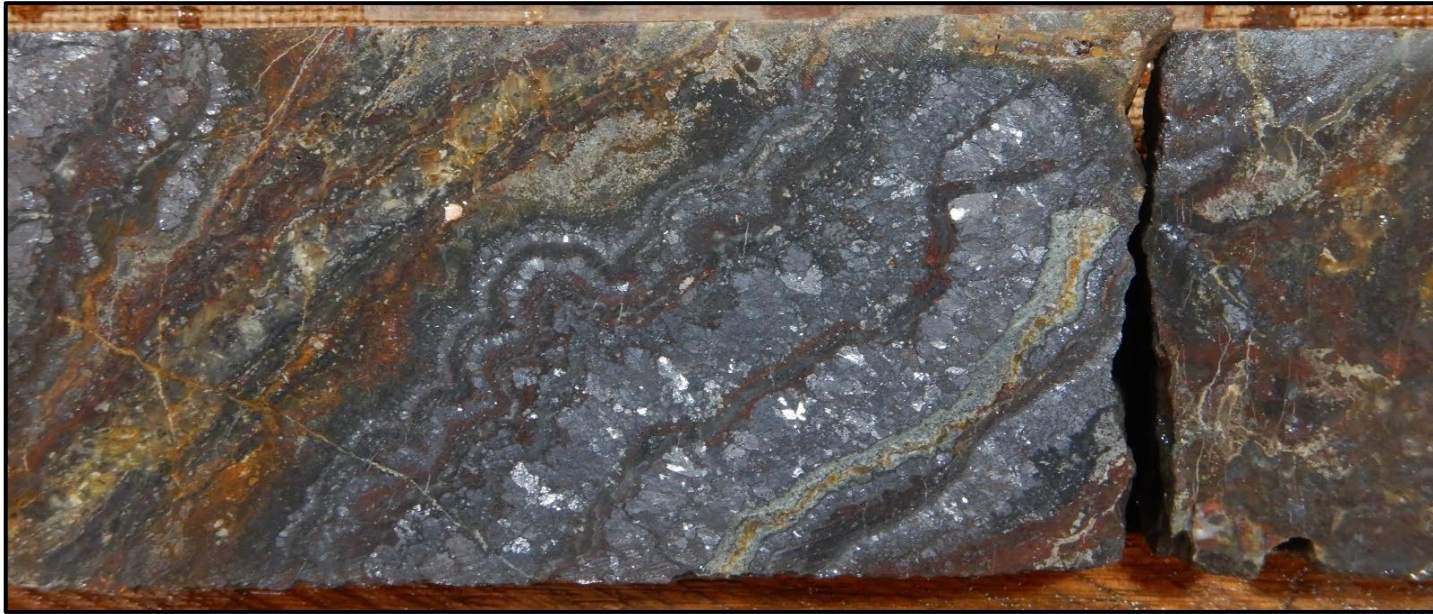
MR-DDH-003: quartz vein with banded and cockade textures. Massive galena bands in the center.
