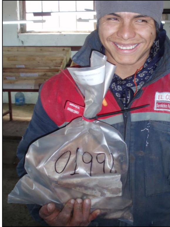
Figure 11-1. Example of security-sealed sample bag ready for sacking and shipping.
