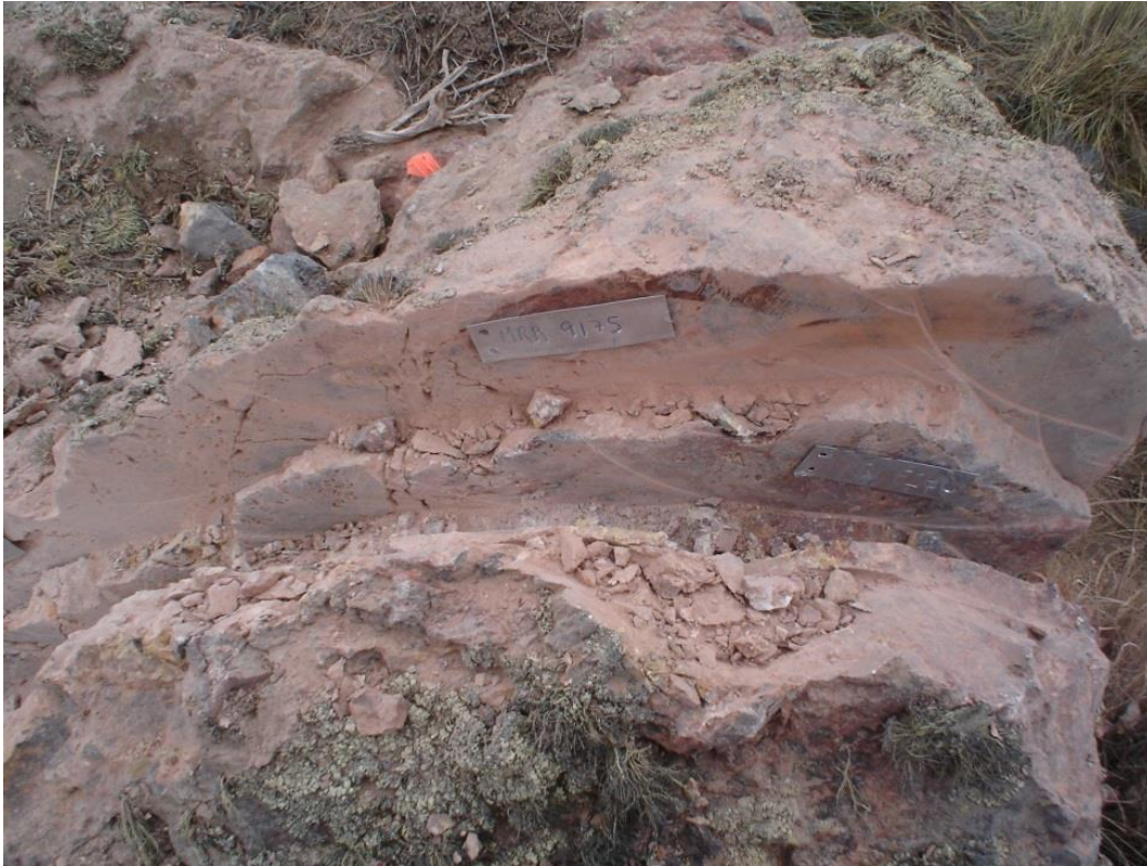
Figure 9-2. Example of Channel Sampling Methods.
