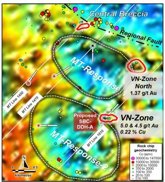
Sobek Central – airborn Mobile MT geophysical survey responses with new drill target
