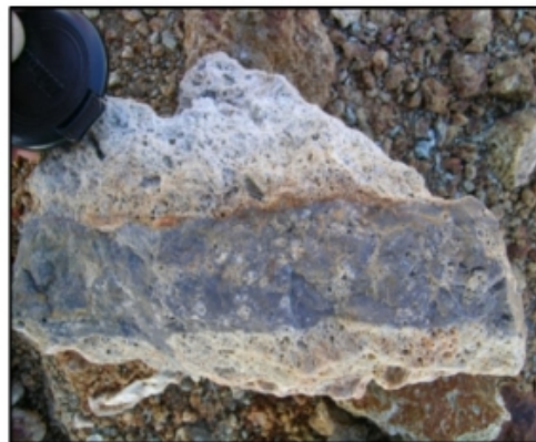
Silver rich chalcedonic veinlets hosted by pyroclastic volcanics underlying the rhyolitic flow dome, maximum assay result 0.06 g/t Au and 193 g/t Ag
