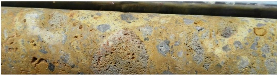
414m (2.54 g/t Au & 1.1 g/t Ag), “Yellow” polymict hydrothermal breccia jarosite-alunite-barite-filled matrix with sub angular vuggy silica altered fragments
