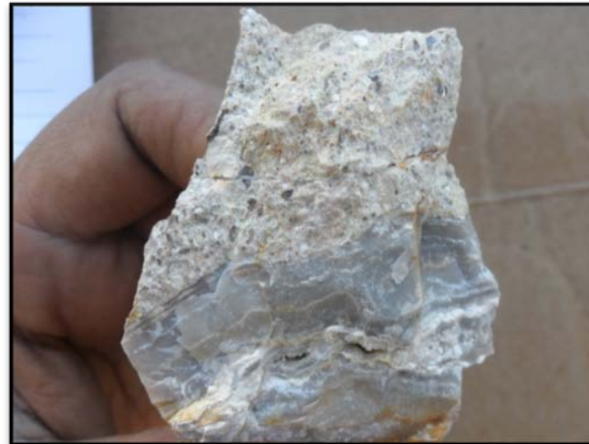
Same structure as previous photo, banded chalcedonic silica veinlet (with adularia) in silicified crystal tuffs, assays to 3.10 g/t Au
