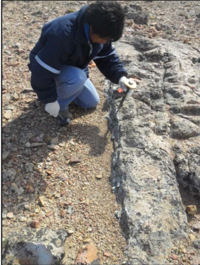
Parallel epithermal veinlets up to 10 cm wide (sheeted veins) crosscutting silicified rhyolitic tuff, Select rock chip samples assayed up to 5.33 g/t Au
