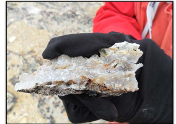
Crystal tuffs with banded chalcedonic silica veinlets with up to 15 cm thick, assays to 5.33 g/t Au
