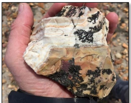
Colloform banded epithermal veinlet cross cutting the Cerro Chato silica
