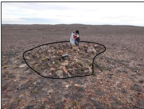
Target 4 - Large clast of altered volcanic wall rock with colloform veining, assays to 12.9 g/t Au and 64.2 g/t Ag
