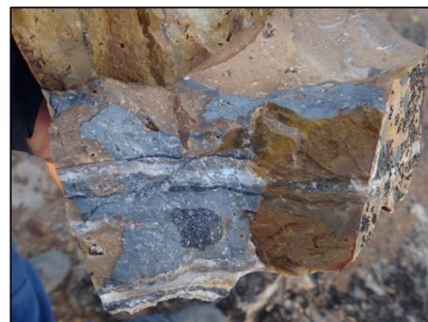
Target 2 – silicified volcanic clasts with colloform saccharoidal & grey pyritic chalcedony, assays to 1.93 g/t Au and 153.6 g/t Ag
