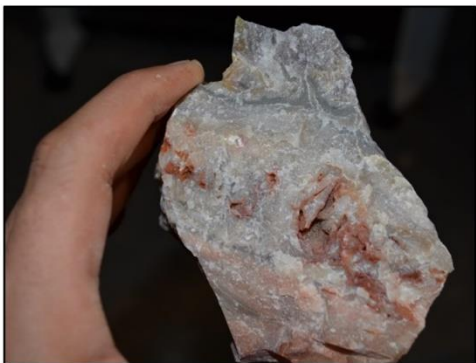
Subangular clasts of banded saccharoidal quartz veins with pulse of dark grey bands of chalcedonic silica, assays to 15.22 g/t Au and 36.40 g/t Ag
