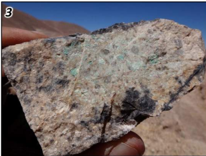
3 Base of rhyolitic pyroclastic altered cap rock with strong silicification, copper & manganese oxides, 4,640 ppm Cu
