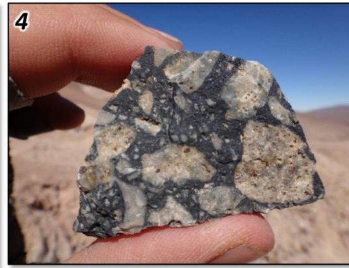
4 Matrix supported tourmaline breccia with silica- diaspore altered welded pyroclastic clasts
