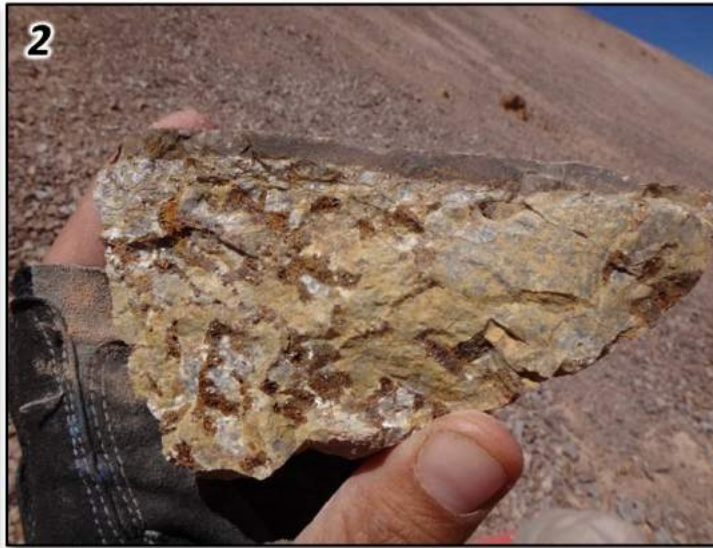
2 Hydrothermal brecciated rhyolitic quartz-eye pyroclastic with crystalline jarosite matrix from the “Lithocap” area
