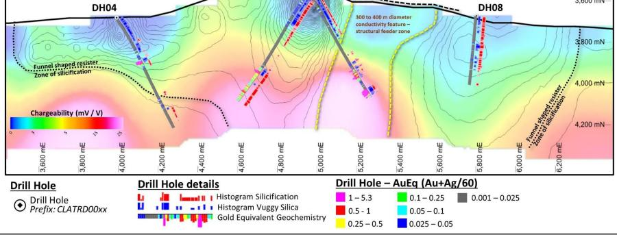
Figure 2 – Atlas Project – Drill results on IP geophysical VOXEL model 52,040E cross section. April 2016.
