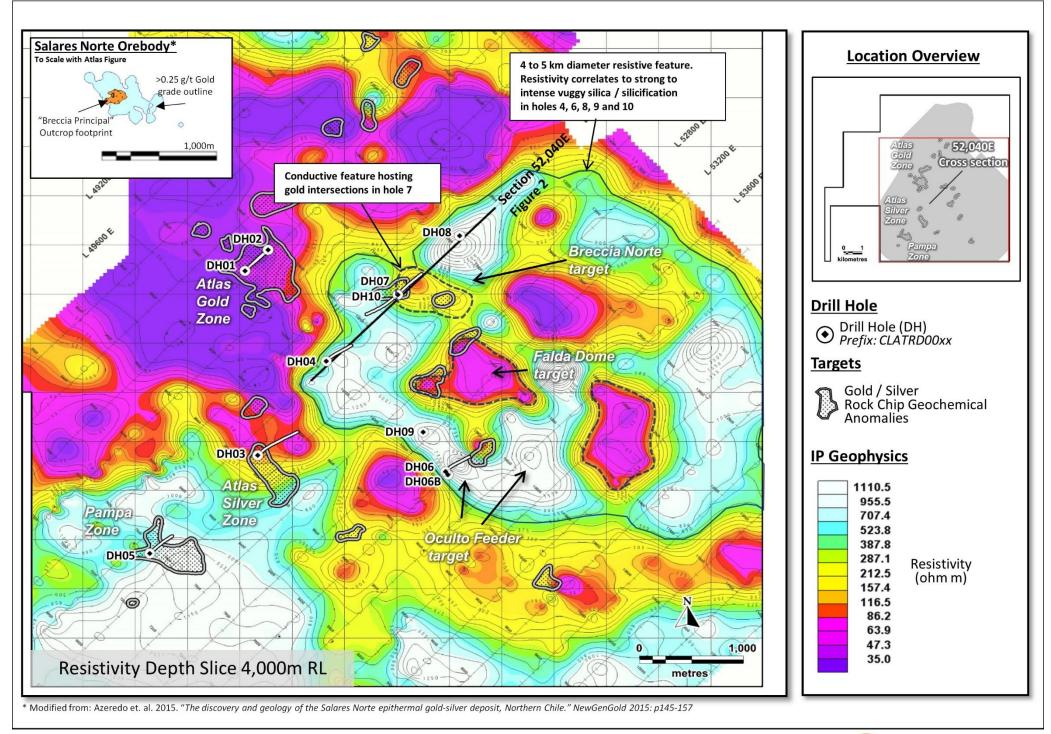
Figure 1 – Atlas Project – Drill hole locations on 4,000m RL IP geophysics depth slice. April 2016.
