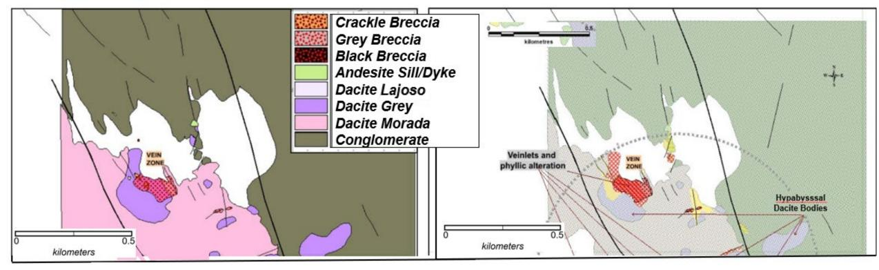
→ Preliminary mapped geology and structural interpretation, occurrence of veinlets and argillic/phyllic alteration. Possible large circular feature associated with the dacitic hypabyssal intrusive bodies.
