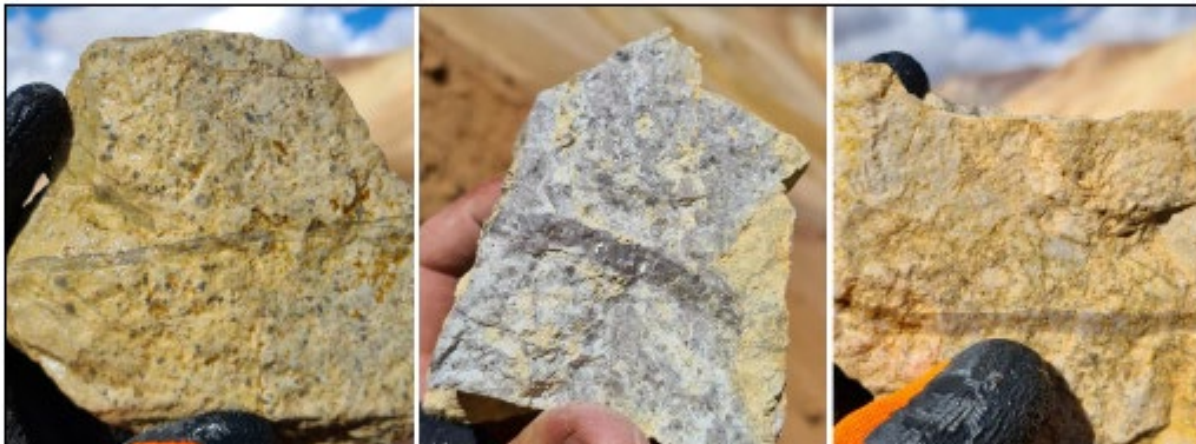
Choiyoi Group Rhyolites and tuffs with Qtz-Ser-Py (Phyllic) alteration and B-Type veinlets (Qtz-Mo)
