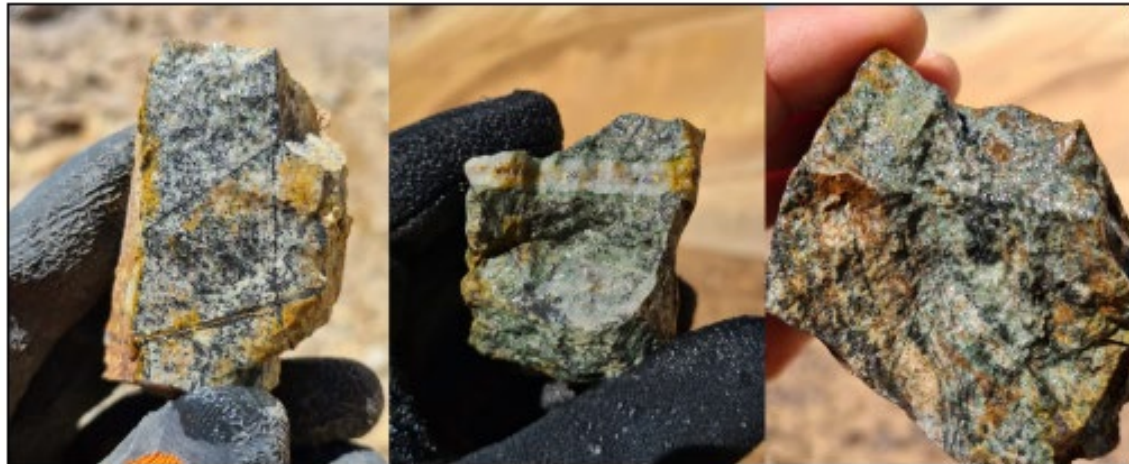
Early Mineral Porphyry with qtz-Magnetite veinlets, potassic alteration and insitu Cu-oxides
