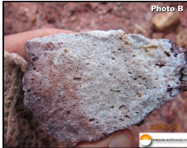
Vuggy silica after porphyritic andesite with up to 7.28 g/t Au & 5.77 g/t Ag
