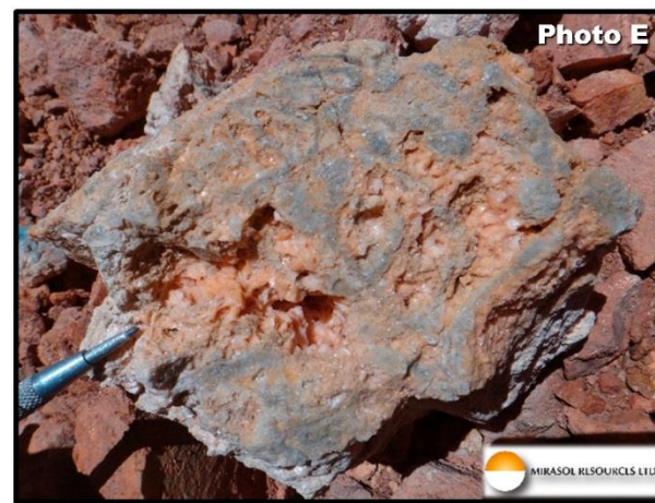
Breccia vuggy silica clasts re-brecciation and leach clasts with late fill of pink alunite, up to 5.07 g/t Au & 7.95 g/t Ag in TR-02
