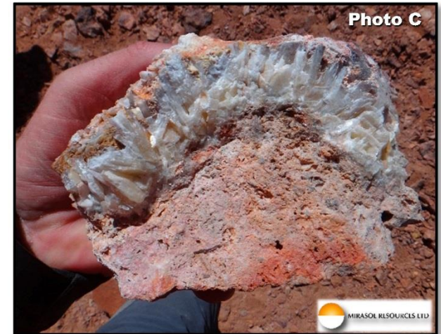
Late stage barite vein common in vuggy silica structures from 3.27-8.85 g/t Au
