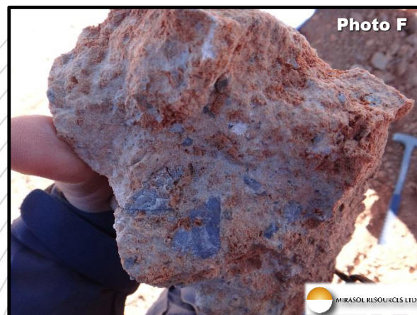
Polyolithic hydrothermal breccia silicified clasts with fine dark sulfides, assays up to 144.7 g/t Ag
