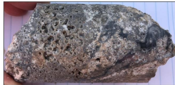
Hole CLATDH0015 - 423.5 m 3.07 g/t Au and 2.1 g/t Ag Phreatomagmatic breccia altered to coarse vuggy quartz. Vugs partially filled by coarse-grained alunite and late pulse of massive fine-grained grey chalcedony.
