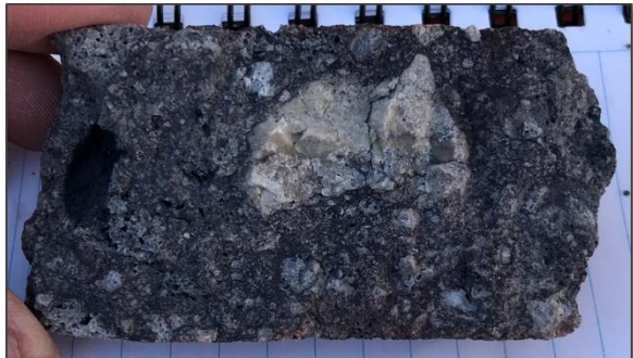
Hole CLATDH0015 - 330.3 to 334 m 0.41 g/t Au and 0.7 g/t Ag Breccia leached vuggy textured quartz matrix with crystalline alunite and late iron oxide (hematite?)/hydroxide.
