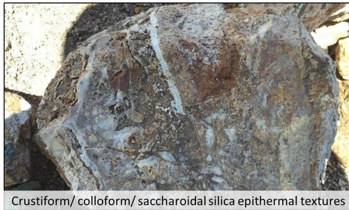
29.6 g/t Au & 16.45 g/t Ag. Banded saccharoidal qtz, clots of Fe oxides, disseminated sulphides
